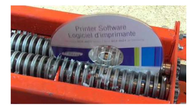
The only way to fully ensure that data cannot be recovered from a hard drive is to carefully shatter the platters with a hammer and safely dispose of the pieces. To destroy software media (floppy disks and CDs), use a shredding machine designed for shredding these materials.
